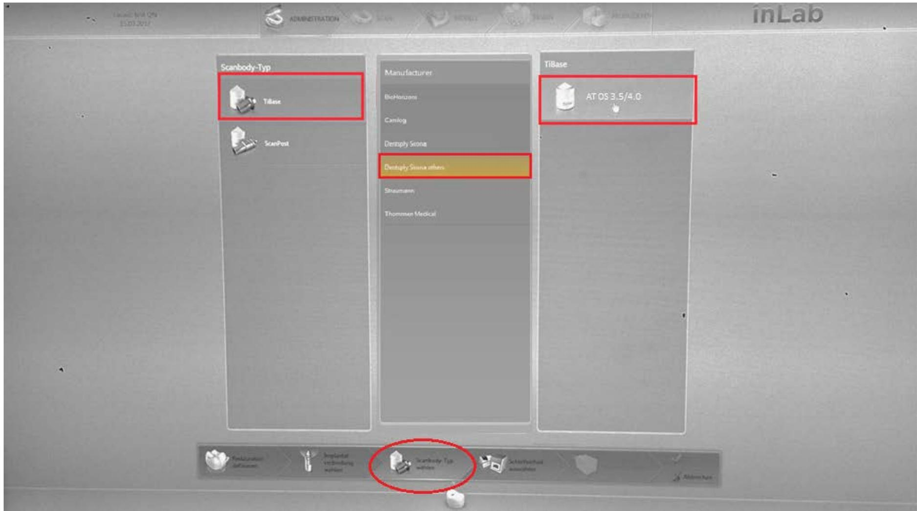
For the **Ti base CEREC® BioniQ QN (Ref. No. 2198.00)** select: Scanbody Type → **TiBase**
